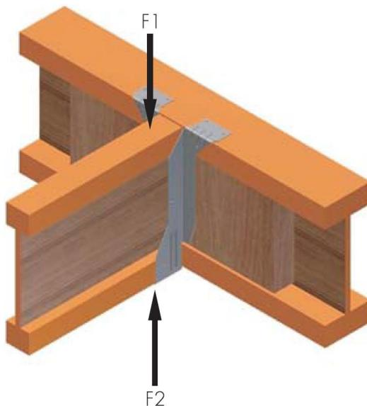
Figure C.1 – Definition of force directions.
