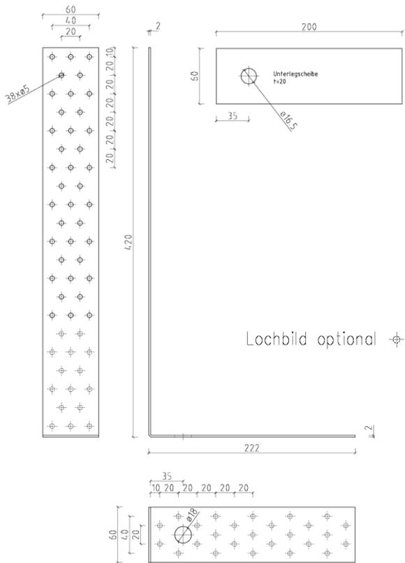
Figure B. 14 Dimensions of type 420x222x60x2,0
