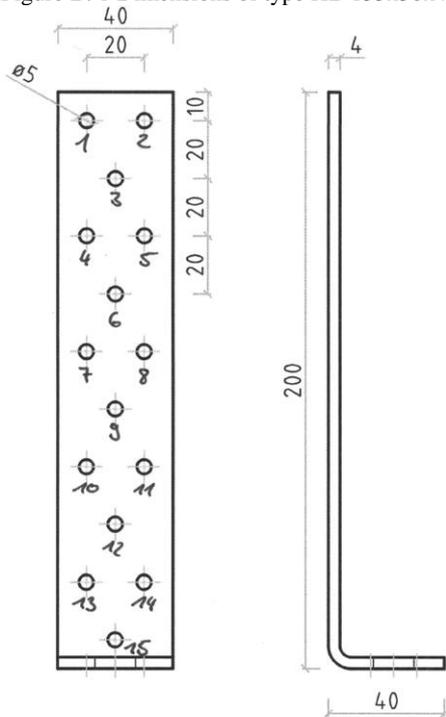
Figure B. 3 Dimensions of type HSB 200x40x40x4,0
