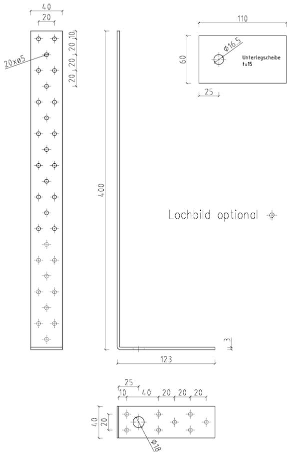
Figure B. 13 Dimensions of type 400x123x40x3,0
