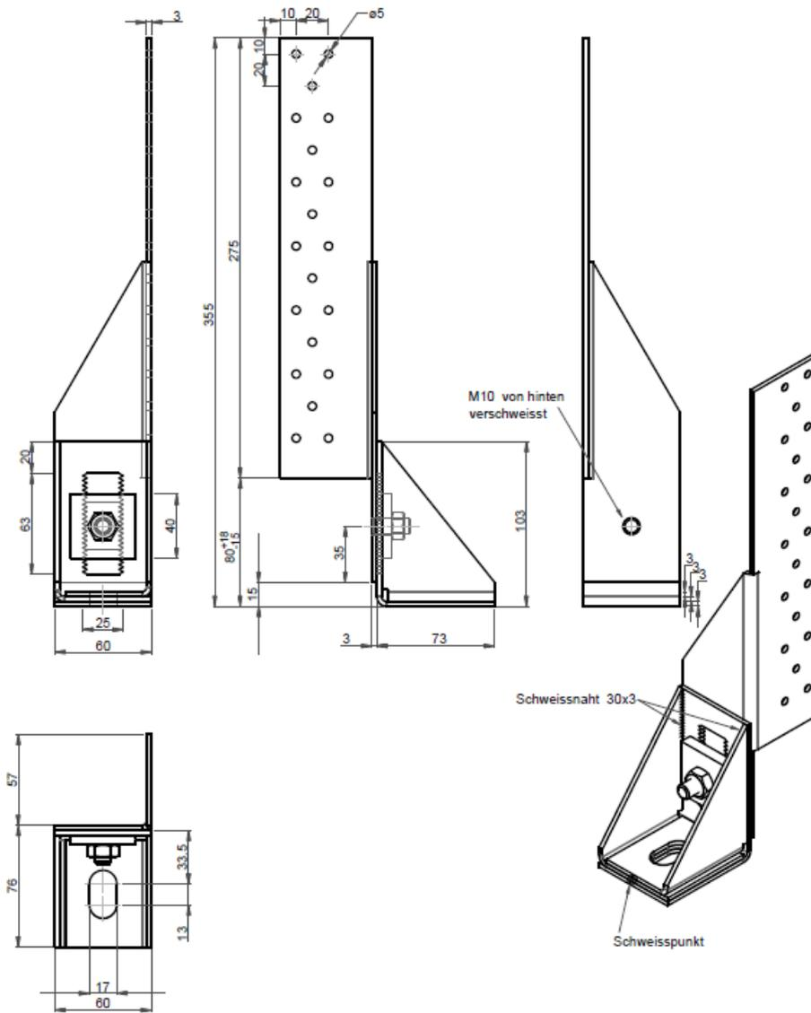
Figure B.44 HT2-RV-340-Stegwinkel-Z-225
