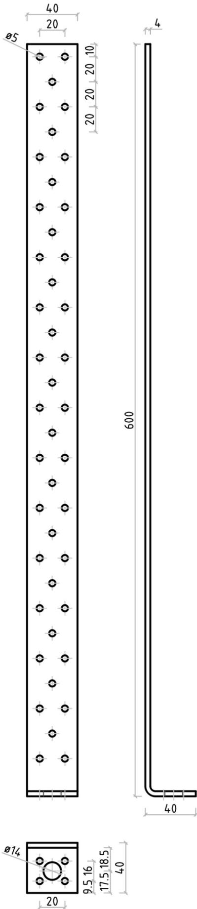
Figure B. 11 Dimensions of type HSB 600x40x40x4,0
