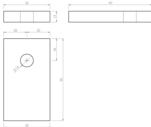
Figure B. 25 Dimensions of washer for hold-downs 142x93x60x2, 280x122x40x2
