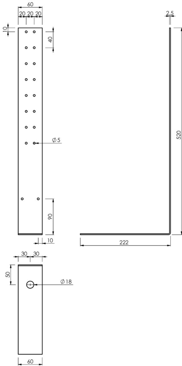
Figure B. 19 Dimensions of type 520x222x60x2,5
