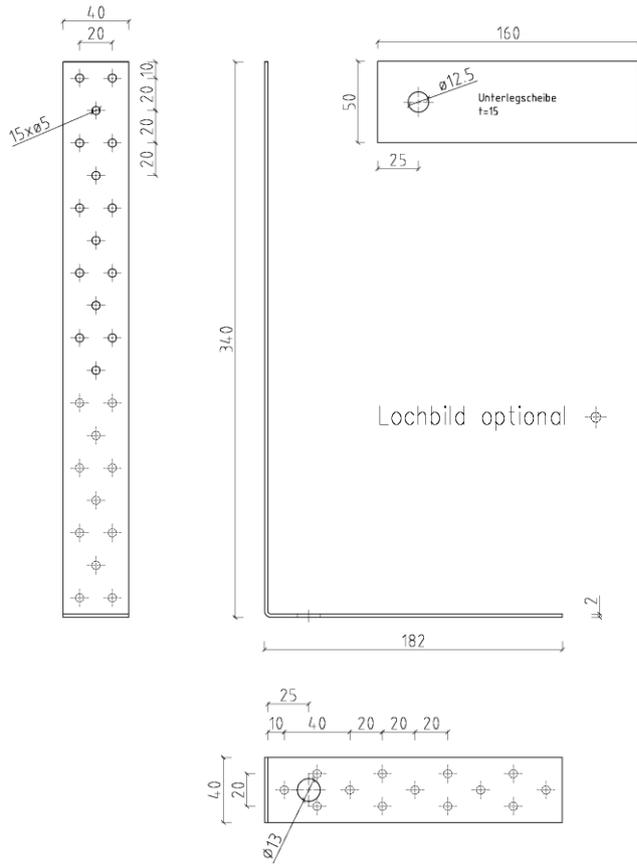
Figure B. 12 Dimensions of type 340x182x40x2,0
