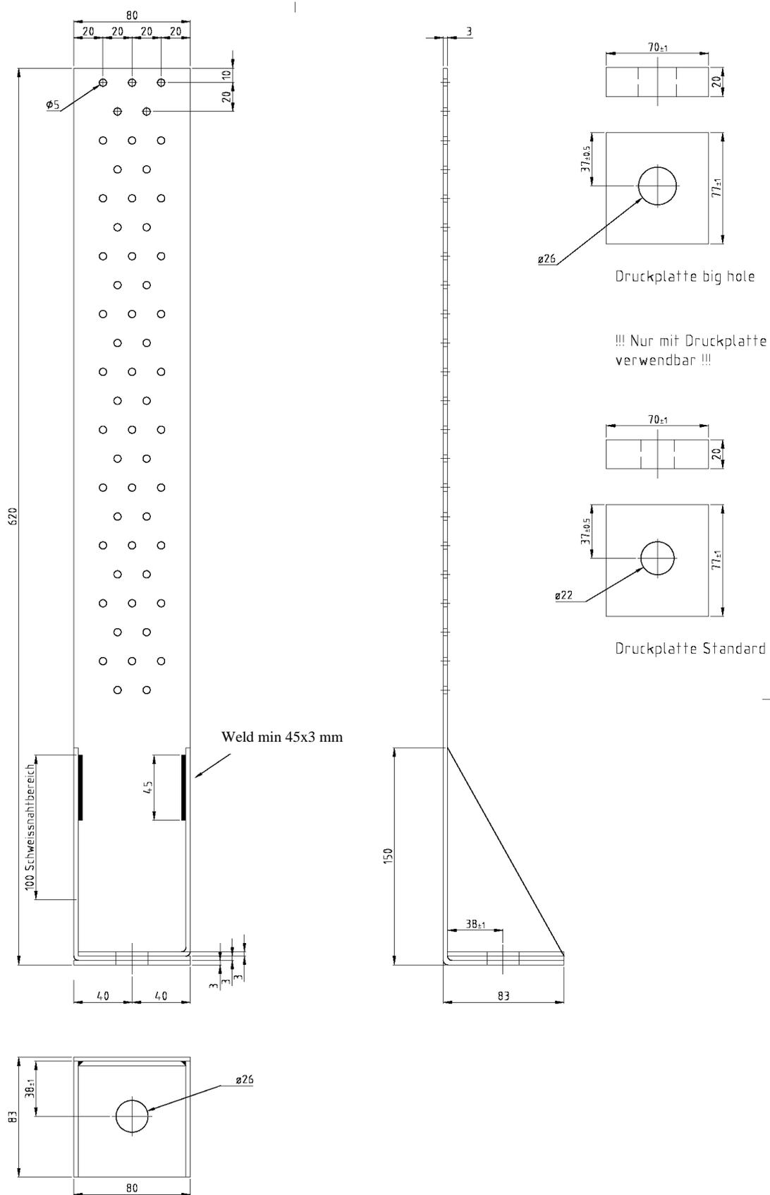
Figure B. 34 Dimensions of type GH HT34 80/620 Big hole (with washer 77x70x20xØ22 or 77x70x20xØ26)
