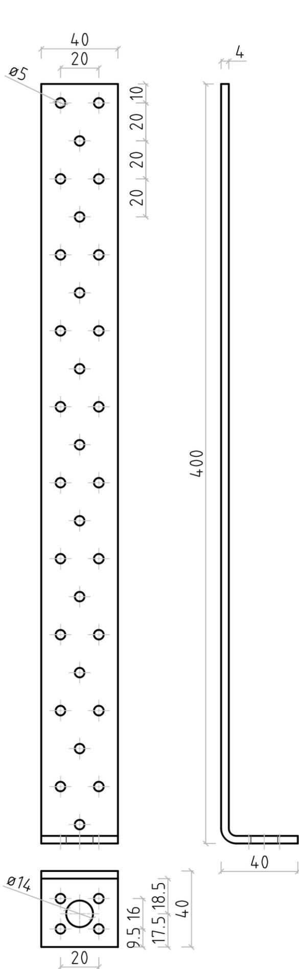
Figure B. 7 Dimensions of type HSB 400x40x40x4,0
