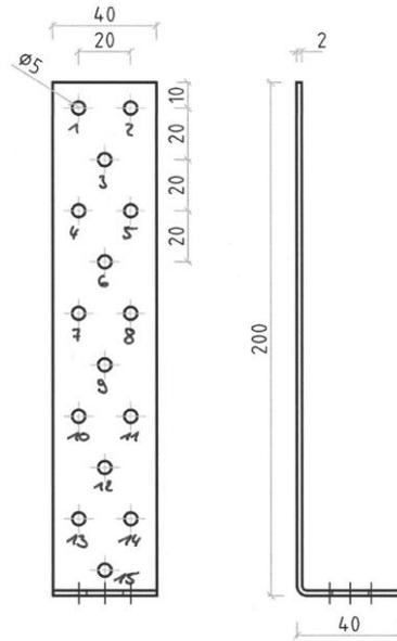
Figure B. 2 Dimensions of type HSB 200x40x40x2,0
