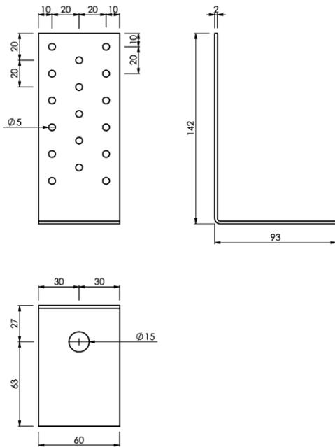
Figure B. 18 Dimensions of type 142x93x60x2
