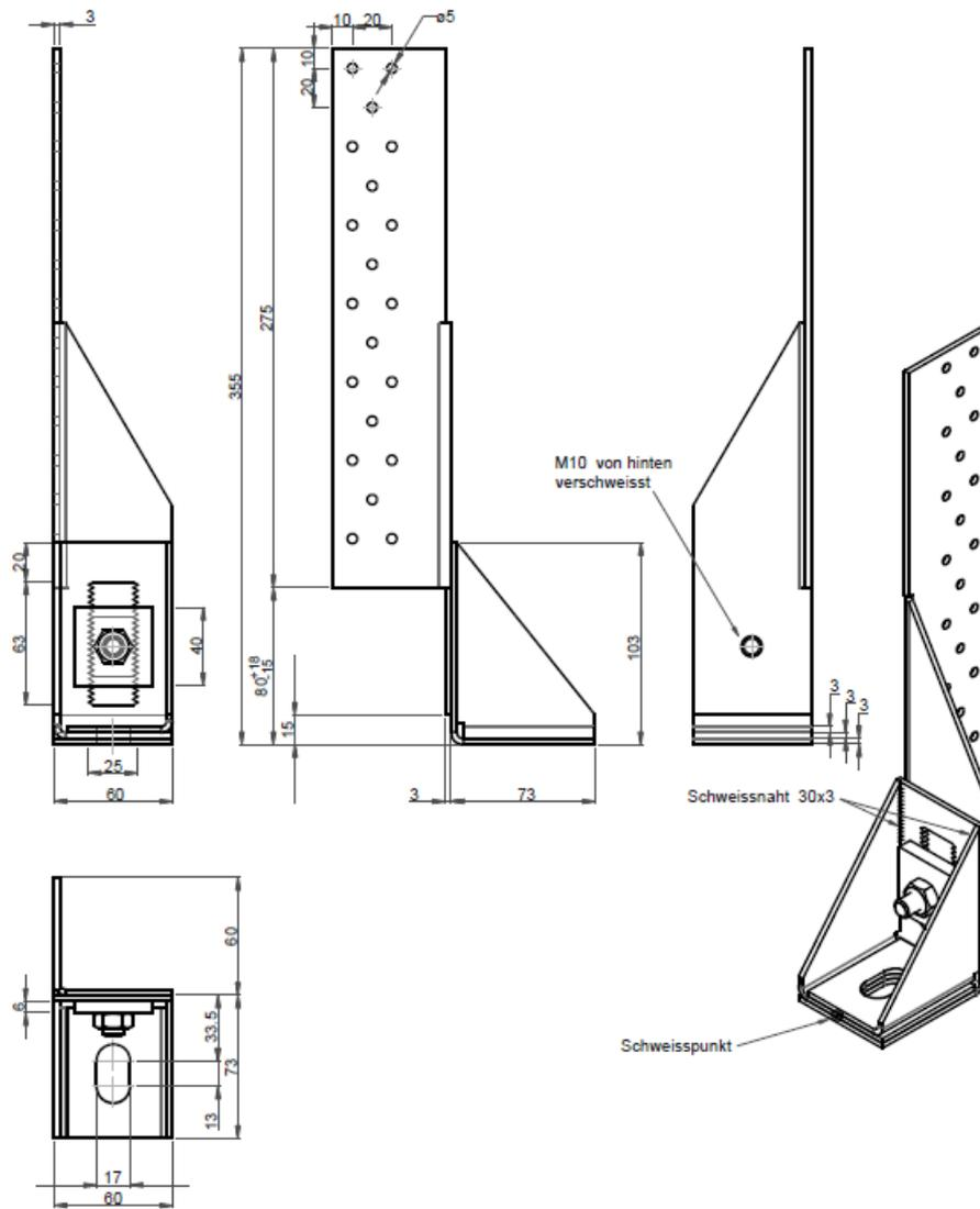
Figure B.42 HT2-LV-340-Stegwinkel-Z-220
