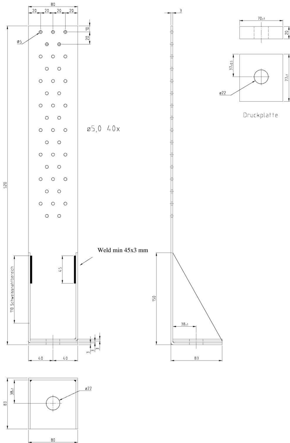
Figure B. 31 Dimensions of type GH HT32 80/520 (drawing with washer 77x70x20)
