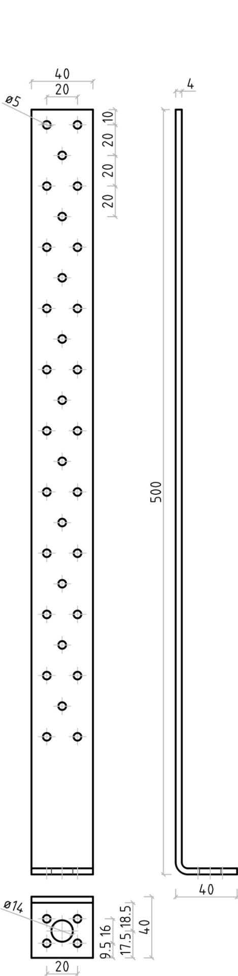
Figure B. 9 Dimensions of type HSB 500x40x40x4,0
