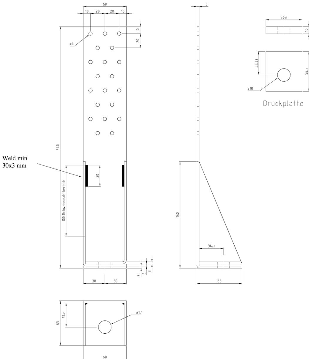
Figure B. 27 Dimensions of type GH HT16 60/340 (drawing with washer 56x50x10)
