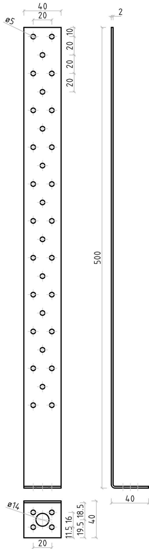
Figure B. 8 Dimensions of type HSB 500x40x40x2,0
