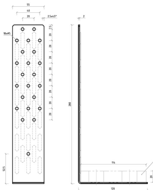
Figure B. 21 Dimensions of Top Vario 280x120x55x2,0
