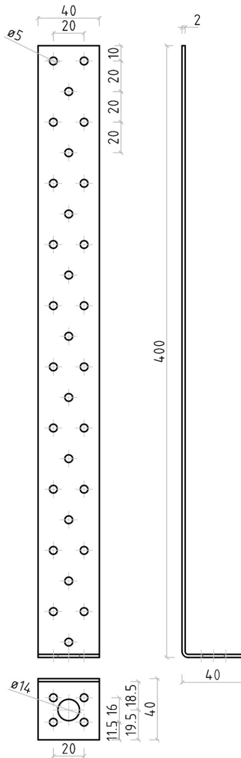
Figure B. 6 Dimensions of type HSB 400x40x40x2,0
