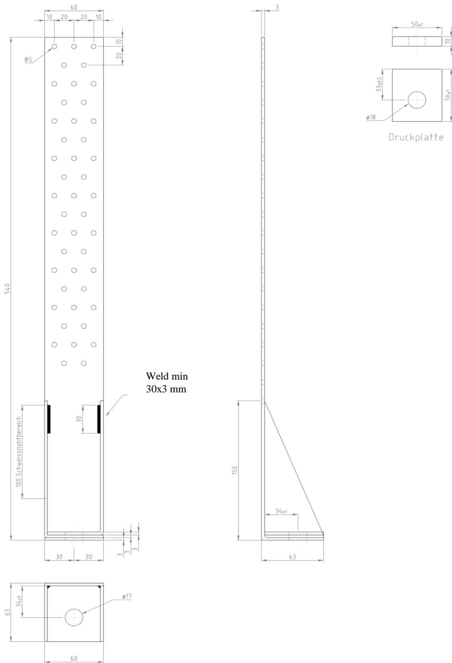
Figure B. 29 Dimensions of type GH HT28 60/540 (drawing with washer 56x50x10)
