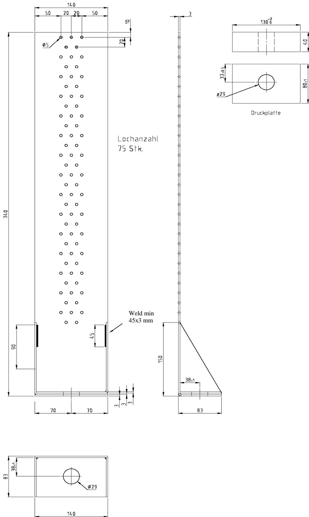
Figure B. 35 Dimensions of type GH HT36 140/740 (drawing with washer 80x130x40)
