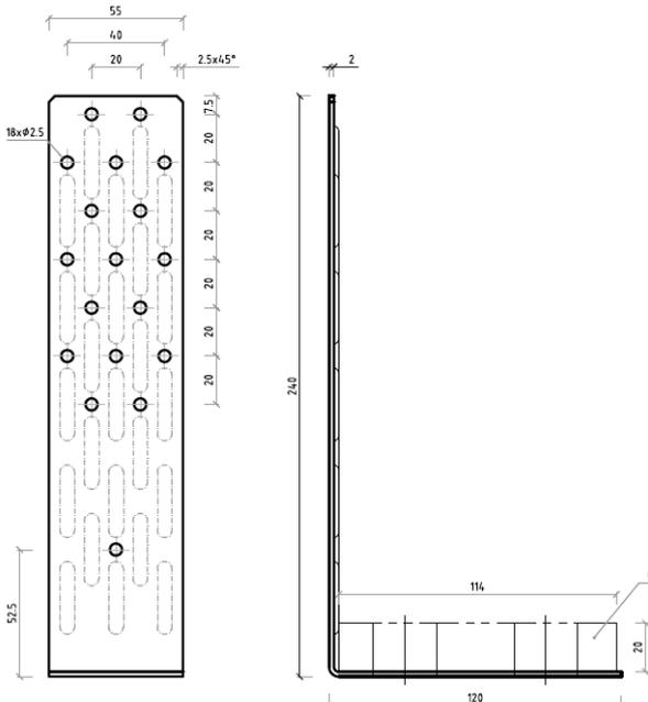
Figure B. 20 Dimensions of Top Vario 240x120x55x2,0
