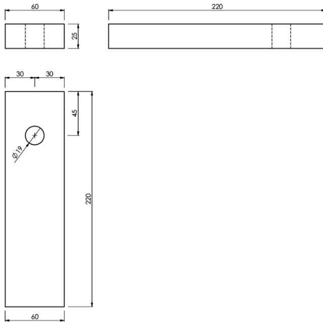
Figure B. 24 Dimensions of washer for hold-down 520x222x60x2,5
