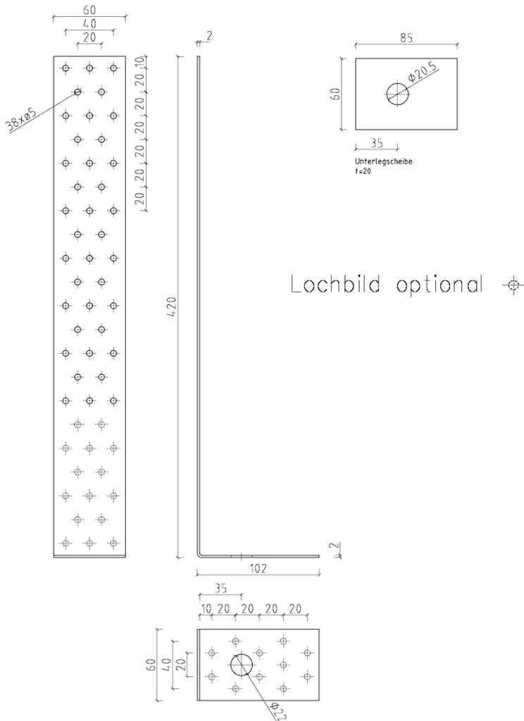
Figure B. 15 Dimensions of type 420x102x60x2,0
