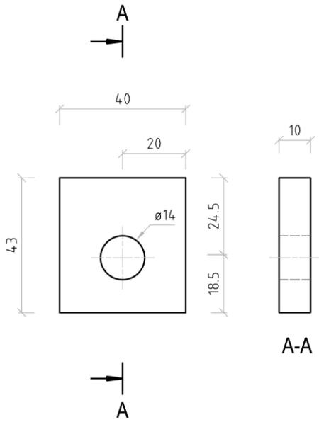
Figure B. 26 Dimensions of washer for type HB and HSB
