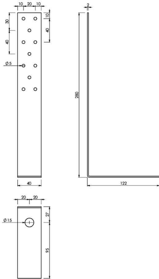
Figure B. 17 Dimensions of type 280x122x40x2
