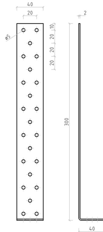
Figure B. 4 Dimensions of type HSB 300x40x40x2,0
