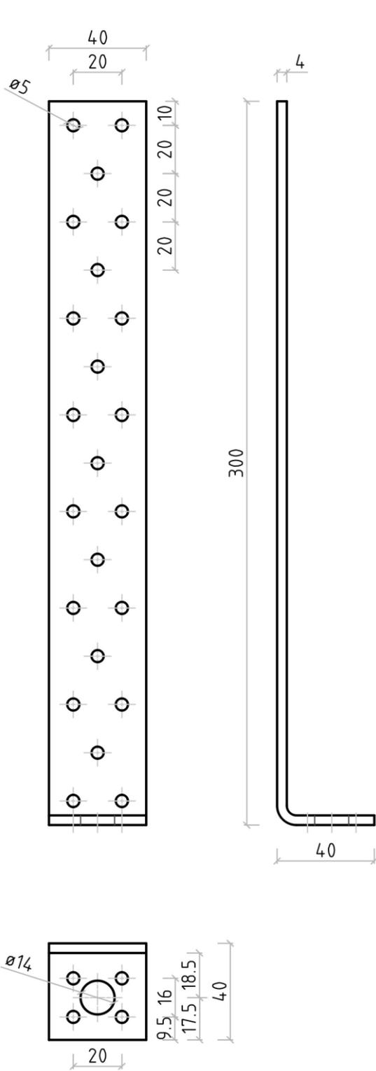
Figure B. 5 Dimensions of type HSB 300x40x40x4,0
