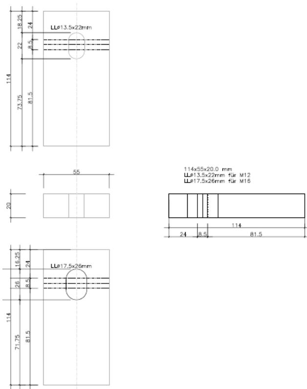
Figure B. 22 Dimensions of washer for Top Vario
