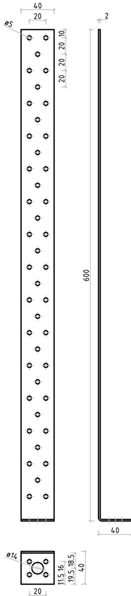
Figure B. 10 Dimensions of type HSB 600x40x40x2,0
