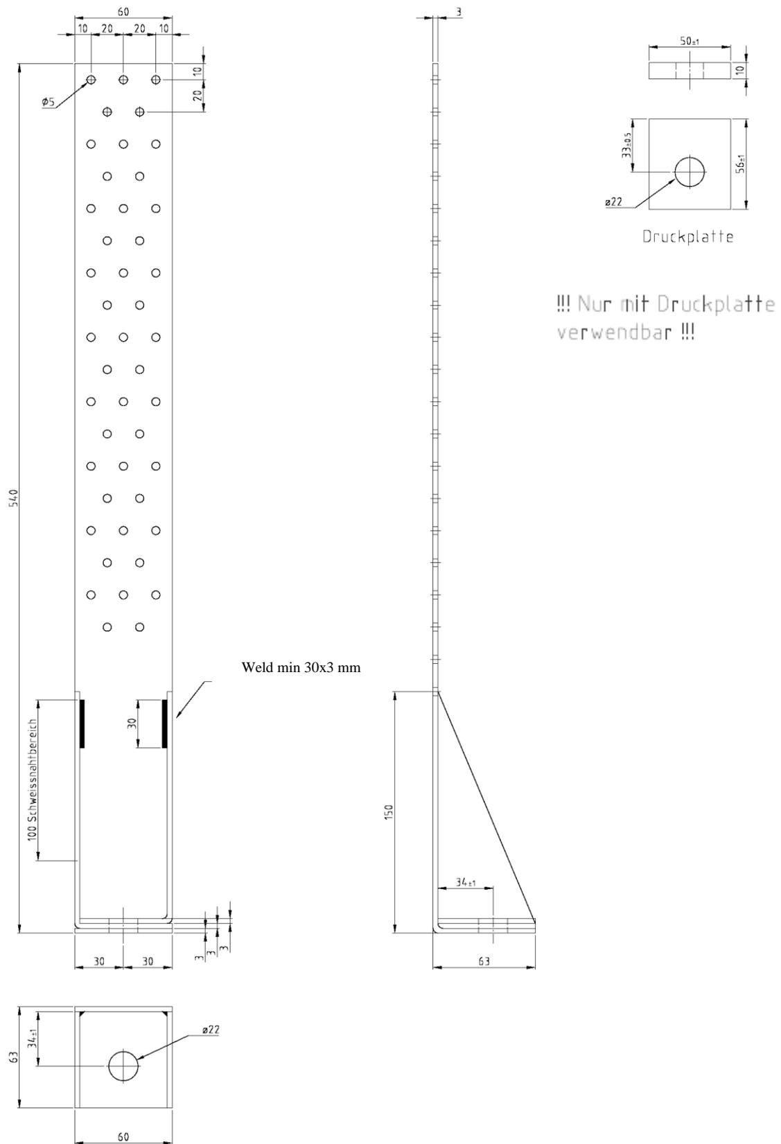
Figure B. 33 Dimensions of type GH HT28 60/540 Big Hole (with washer 56x50x10)
