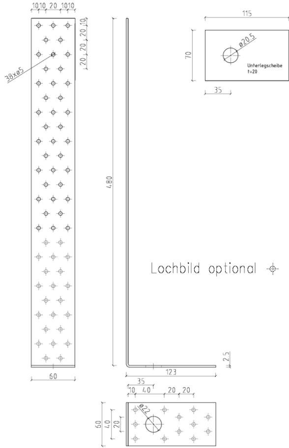
Figure B. 16 Dimensions of type 480x123x60x2,5
