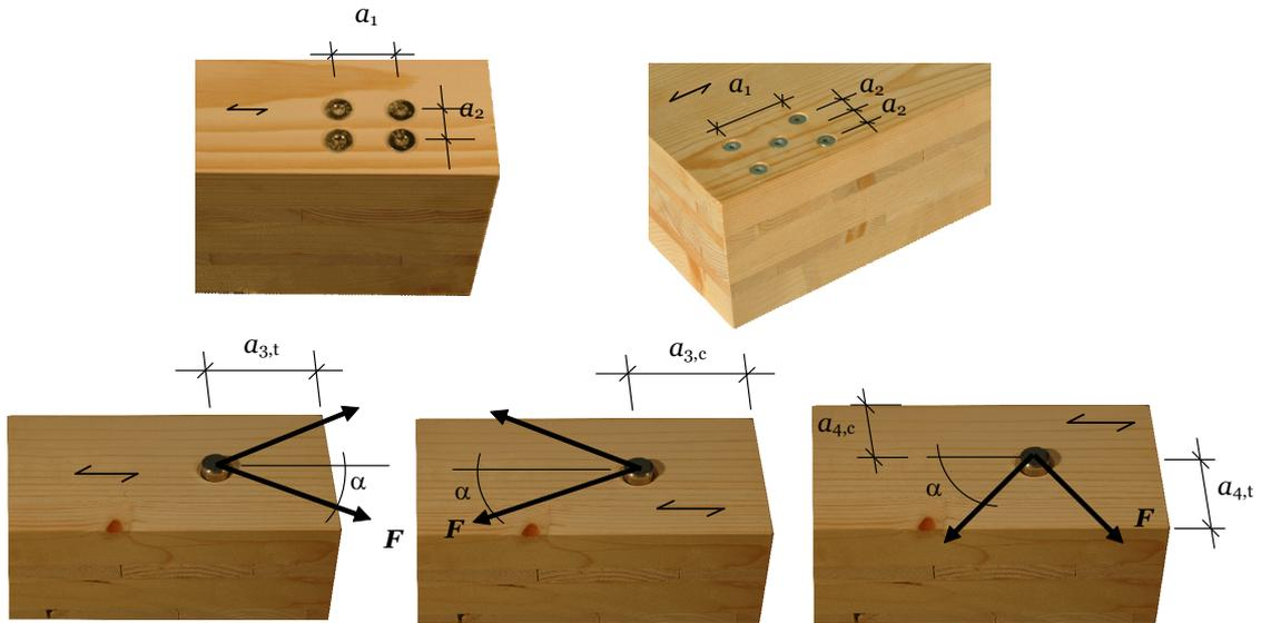
Figure 2: Definition of spacing, end and edge distances in the edge surface unless otherwise specified in the technical specification (ETA or hEN) for the cross laminated timber:
