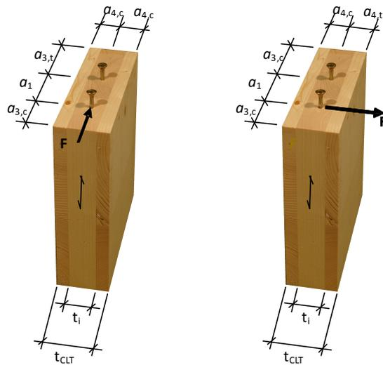
Minimum distances and spacing for screws in the plane surface (wide surface) or edge surface of cross laminated timber
